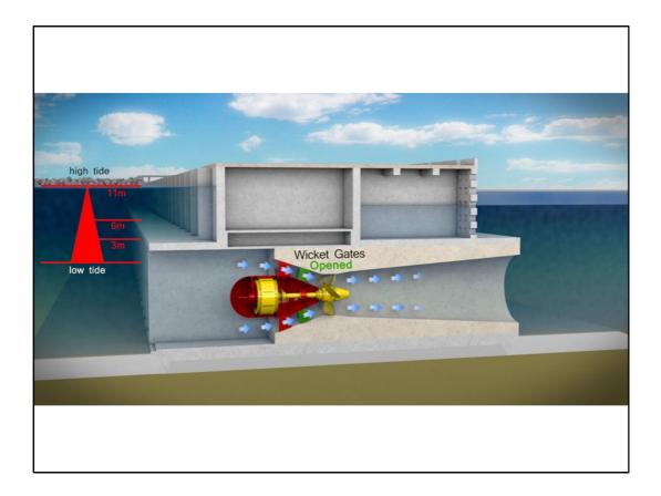
The lagoons operate on a simple basis. As the tide rises, water flows in and turns the turbine. As it falls water flows out and turns it again.
