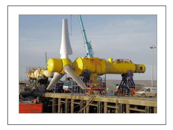
And here is the first of four turbines to be installed in the Sound of Islay, between Jura and Islay. When complete in 2023 this will be the largest tidal power scheme in the world, and by 2022 Scotland should have 640MW of tidal current power coming onstream.
