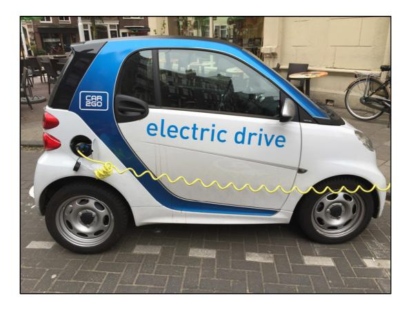
Electric Vehicles have just 20 moving parts, and their motors are around 90% efficient. ICEs have 2000 moving parts and are around 30-40% efficient.
