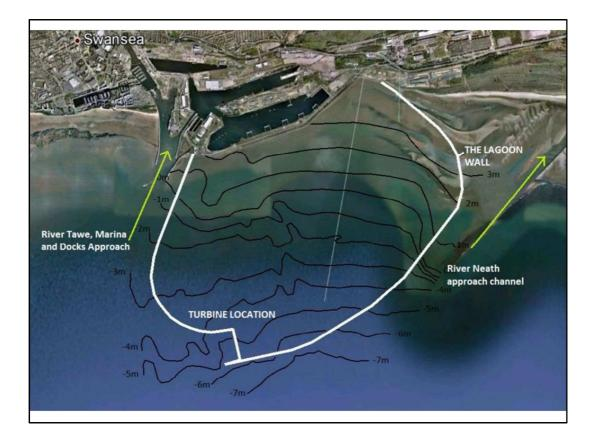
It's not going to be all solar PV in the UK, that's for sure! We have 5 times less solar energy in winter time than in summer, so our challenge is to store energy for the winter. This is a diagram of the Swansea tidal lagoon, which has been given the go-ahead. It is a prototype for 9 other possible lagoons in the Bristol Channel, which has the second highest tides in the world.
